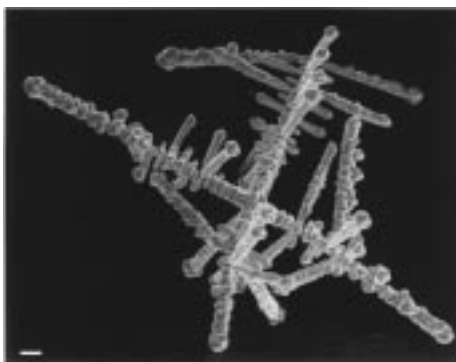
Figure 2. AgBr crystallized from DMSO/9% PVC in the two-phase (gel/liquid) configuration. Scale bar, 10 \mu\text{m} .
